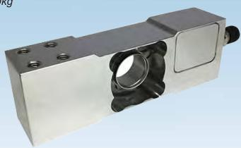
The T12D digital stainless steel single-point load cell is ideal for high resolution, high-speed weight measurement with off-centre loads in challenging applications. It provides a direct output in weight units, such as kg, that can be connected to a PLC without any additional transmitter, amplifier or indicator. This provides significant cost savings. The direct output is via a CAN bus interface using a CANopen protocol.
